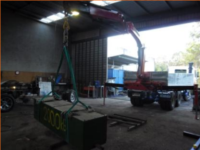
10Yr Refurbishment of Crane
